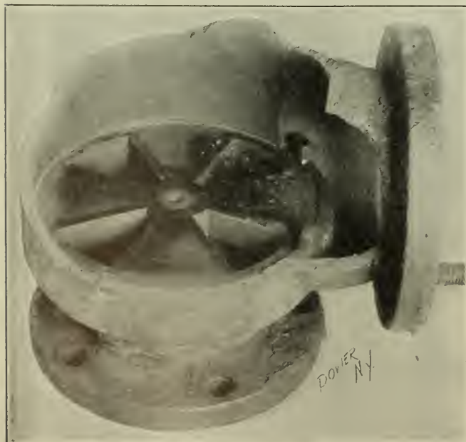
VIEW OF VALVE BODY, SHOWING FRACTURE
